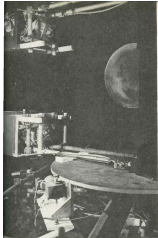
Selsyn driven, rotating plate projectors mounted on "Jupiter machine" rig.
