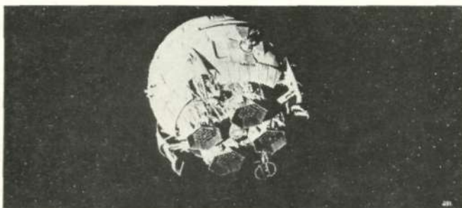
Aires, a globular vehicle which carries passengers from the space station to the Moon has retractable legs that extend for landing.
