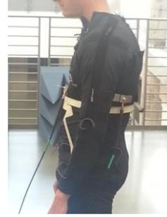
Fig. 4. Around the torso  $S_{21}$  measurement
