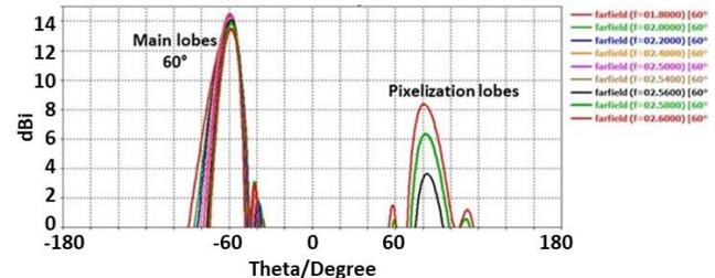
Figure 15: ARMA Radiation pattern evolution as a function of  $\theta$  for different frequencies of the band in the case of a  $60^\circ$  beam-steering.
