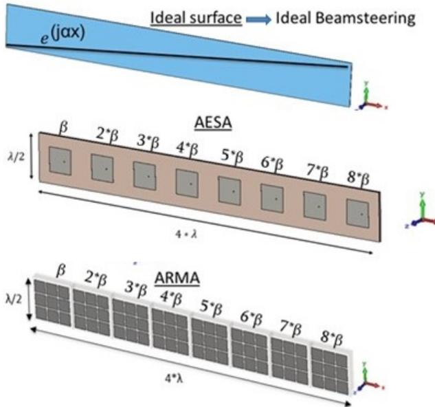
Figure 8: Ideal Beam-steering surface, AESA & ARMA structures.
