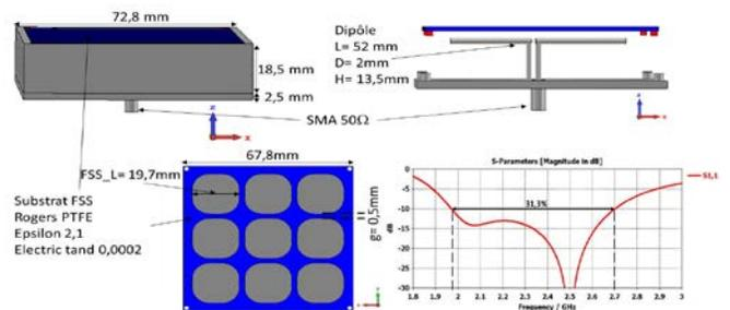
Figure 10: Wide band pixel and S11 parameter as a function of frequency.
