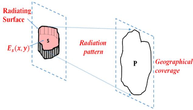
Figure 1: Radiation pattern obtained directly from the radiating surface limited to its upper part.
