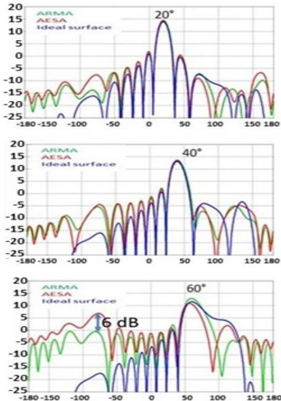
Figure 9: Comparison of ideal surface, AESA and ARMA radiation patterns for a beam-steering procedure in the  $\theta = 20^\circ, 40^\circ$  and  $60^\circ$  directions.
