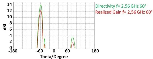
Figure 16: Directivity and Realized Gain comparison for a steering angle of 60° at 2.56GHz.
