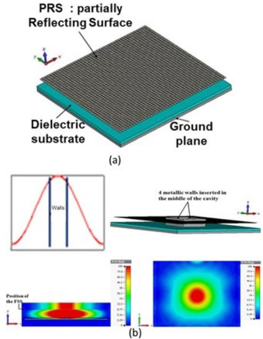
Figure 6: Figure 6 (a) High gain EBG Antenna (b) Vertical metallic walls inside the EBG Antenna and E-field cartography on the radiating surface.
