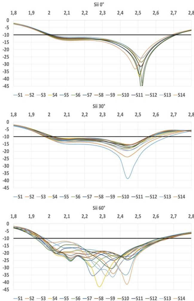
Figure 12:  $S_{ii}$  active parameters evolution as a function of the frequency for a beam-steering procedure in the  $\theta = 0^\circ, 30^\circ$  and  $60^\circ$  directions.
