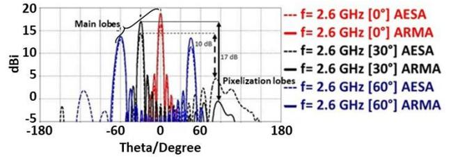
Figure 13: ARMA Radiations patterns evolution as a function of the  $\theta$  for the highest frequencies of the band in the case of a  $0^\circ, 30^\circ$  and  $60^\circ$  beam-steering and comparison with the array approach (dotted curves).
