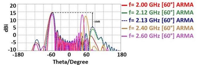
Figure 14: ARMA Realized Gain evolution as a function of  $\theta$  for different frequencies of the band in the case of a  $60^\circ$  beam-steering.
