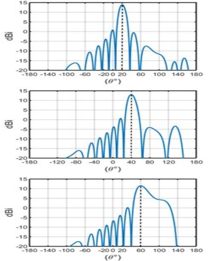
Figure 4: Ideal beam-steering for  $20^\circ$   $40^\circ$  and  $60^\circ$ .
