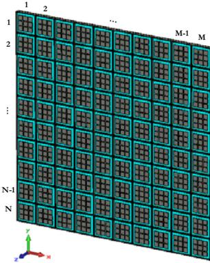
Figure 5: 2D low profile Matrix Antenna called ARMA.
