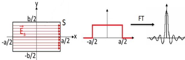
Figure 2: A planar uniform rectangular radiating surface and its FT.
