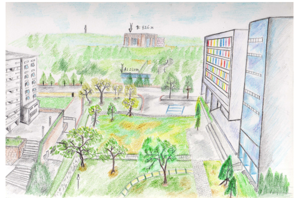
Fig. 25. Aerial perspective of the targets and terrain contour for radar detection; the phased array radar system is located at the ninth floor, Kuang-Fu campus of National Chiao-Tung University, Hsinchu, Taiwan. Notably, target A is a welded wire mesh fence with the mesh size smaller than half wavelength (9410 MHz) .
