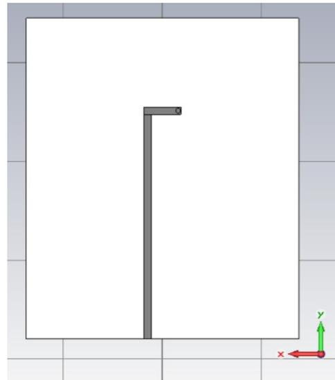
Fig. 13. PCB layout of the printed Yagi antenna employed in the beam-forming array system (bottom layer.)
