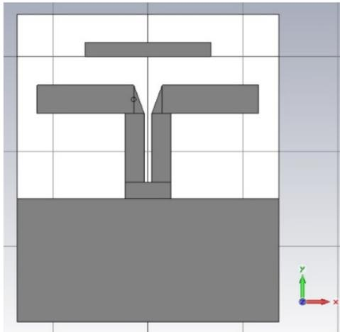
Fig. 12. PCB layout of the printed Yagi antenna employed in the beam-forming array system (top layer).
