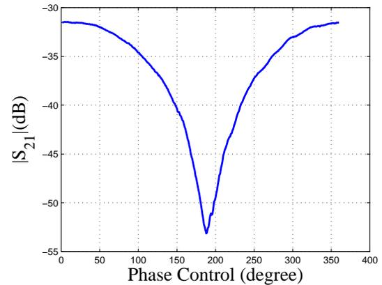
Fig. 5. Measurement of the combined power normalized to the incident power.
