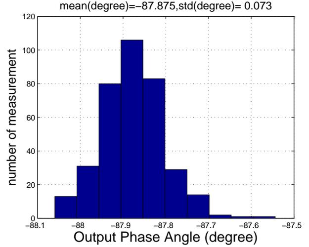
Fig. 9. Histogram of the phase angle measured from vector network analyzer of channel 2; mean and standard deviation are  $-87.875^\circ$  and  $0.073^\circ$ , respectively.
