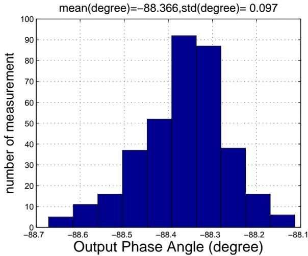
Fig. 11. Histogram of the phase angle measured from vector network analyzer of channel 4; mean and standard deviation are  $-88.366^\circ$  and  $0.097^\circ$ , respectively.
