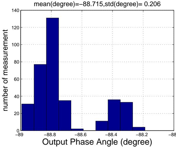
Fig. 8. Histogram of the phase angle measured from vector network analyzer of channel 1; mean and standard deviation are  $-88.715^\circ$  and  $0.206^\circ$ , respectively.
