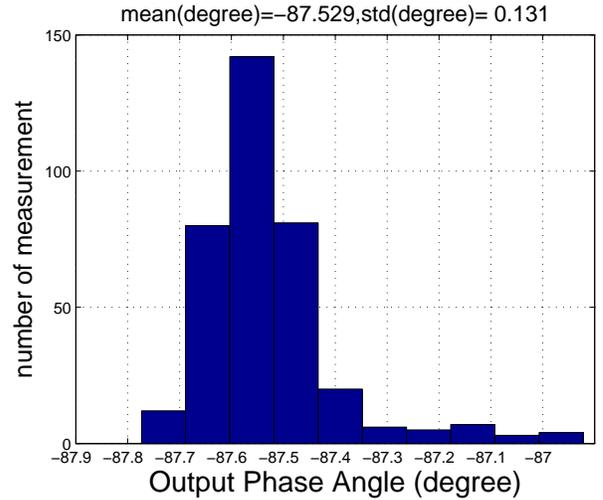
Fig. 10. Histogram of the phase angle measured from vector network analyzer of channel 3; mean and standard deviation are  $-87.529^\circ$  and  $0.131^\circ$ , respectively.
