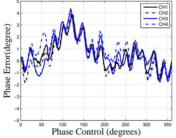
Fig. 2. Measurement of the phase error corresponding to each vector modulator.
