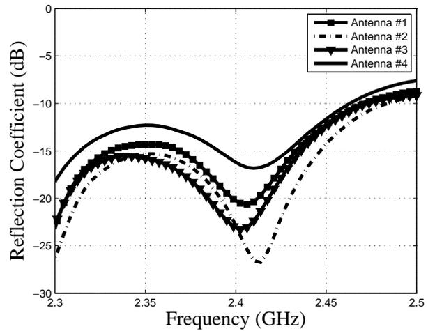
Fig. 14. Measured reflection coefficient of the 4 printed Yagi antennas.
