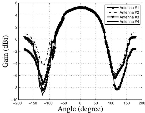
Fig. 15. Measured radiation pattern of the 4 printed Yagi antennas.
