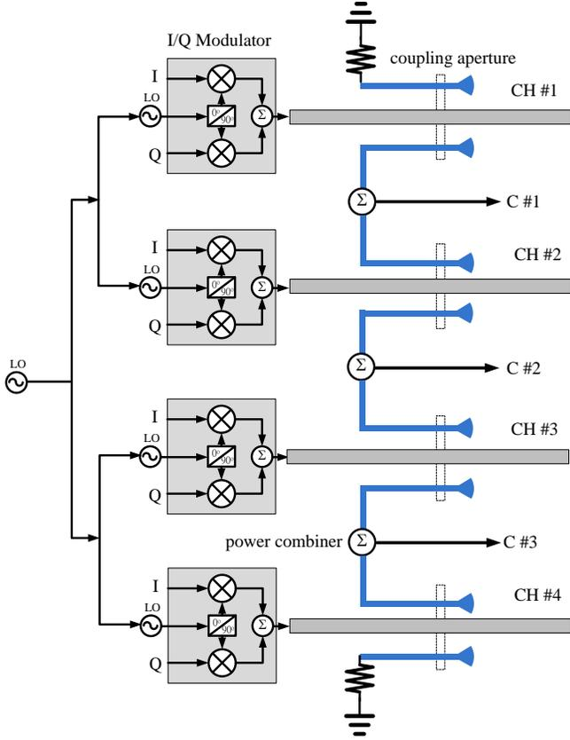
Fig. 1. System block of the 4-channel phase-adjustable local oscillators equipped with the on-board calibration circuit.
