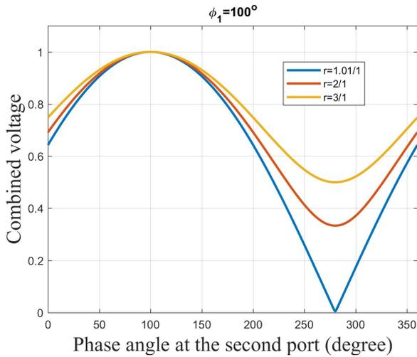
Fig. 3. Combined voltage amplitude at the ideal power combinator against the phase angle at the second port; the phase angle at the first port is assumed to be  $100^\circ$ .
