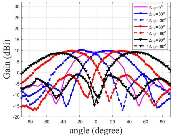
Fig. 16. Measured radiation pattern at 2.4 GHz for various  $\Delta\psi$  of the uniform antenna array fed by the phase-adjustable LO signals
