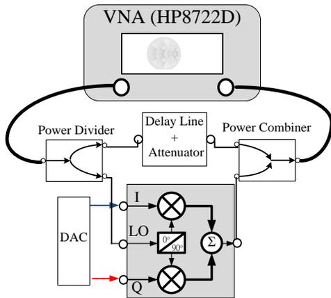
Fig. 4. Experimental setup for proving the power combining mechanism used in phase calibration.
