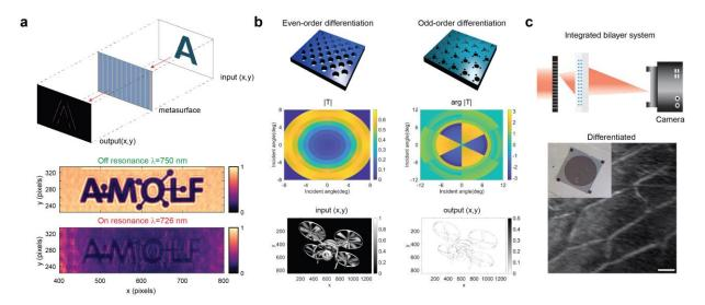
**a**. Top: conceptual schematic of optical computing metasurface. Bottom: experimental second-order image differentiation. Optical microscopy image of the metasurface output for resonant ( $\lambda$  = 726 nm) and off-resonant ( $\lambda$  = 750 nm) illumination.
