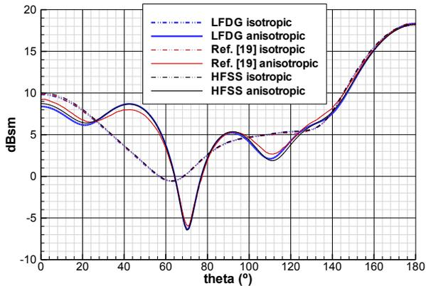
Fig. 9: Bistatic RCS of an isotropic/anisotropic sphere ( $D = 1.2\lambda$  and  $\lambda = 1.0m$ ). LFDG results are compared to those appearing in [167], and computed with Ansoft HFSS.
