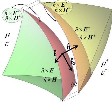
Fig. 1: Notation used for the definition of the numerical fluxes.
