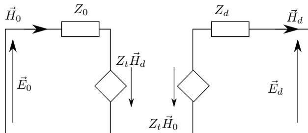
Fig. 11: Magnetic field-controlled circuit representation of a thin layer.
