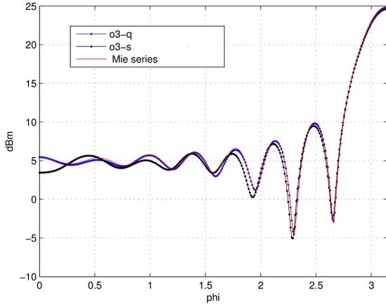
Fig. 5: RCS at 450 MHz of a 1m radius PEC sphere meshed with the same number of linear and quadratic tetrahedrons and a spatial basis of order  $p = 3$ . Results obtained with GEG-UGR SEMBA software ([www.ugrfdtd.es](http://www.ugrfdtd.es)).
