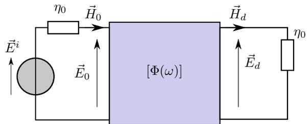
Fig. 10: Two-port representation of the air-embedded panel illuminated by a TEM plane wave.
