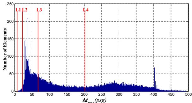
(a) Example of distribution of time steps in a real problem (described in [10]). The choice of the time step and the time steps of different levels have been included in the plot. The estimated average time step was 88.5 ps, compared to the minimum 10.5 ps [12].
