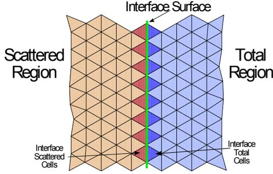
Fig. 7: Scattered field (orange) and total field regions (blue). The elements that need to have altered fluxes are marked in darker colors.
