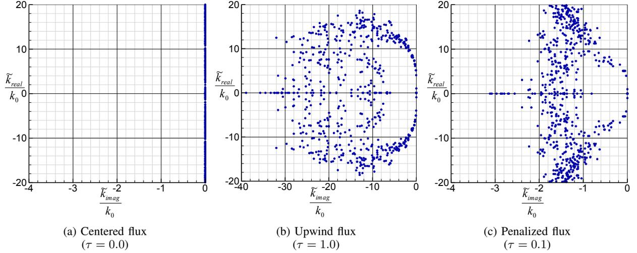
Fig. 3: Normalized spectrum of the DG operator for a cubic domain (meshed with 24 tetrahedrons) with periodic boundary conditions. We can see how the centered flux does not provide an isolated kernel, contrary to the upwind and penalized fluxes.
