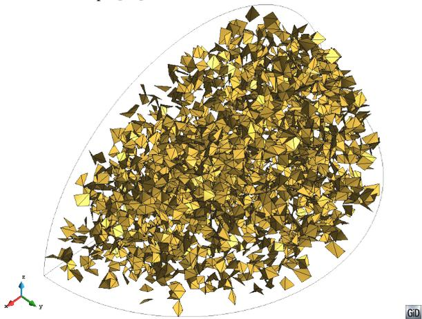
(b) Elements evolved with the doubling of the minimum timestep (Tier 1) using an LTS technique for LF2 [20].
