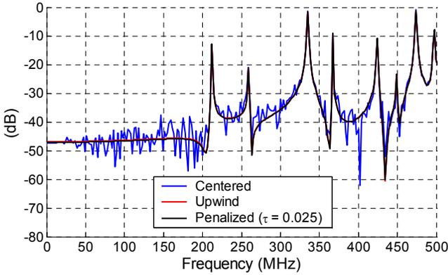
Fig. 2: Power spectrum of the electric field at an arbitrary point inside a 1 m PEC cavity. The effect of the non-attenuation of the centered flux spectrum can be appreciated compared with the upwind and penalized fluxes.
