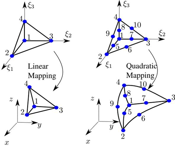
Fig. 4: Mapping from the reference element for linear (first geometrical order) and quadratic (second geometrical order) tetrahedrons.
